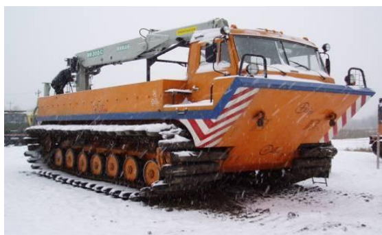
Fig. 27. TTM-6901E. Snow and swamp-going vehicle with an excavator mount
