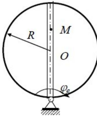
$$S_r = 20 \sin(\pi t/3) \text{ см}, \quad \varphi_e = 6t - 2t^3, \\ t = 0,5 \text{ с}, \quad R = 20 \text{ см}.$$
