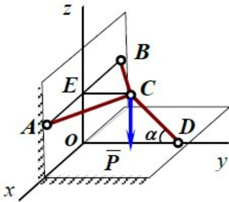
$P = 3 \text{ кН}$ ,  $\alpha = 45^\circ$ ,  $CD \perp Ox$ ,  $BC = AC = 2EC$
