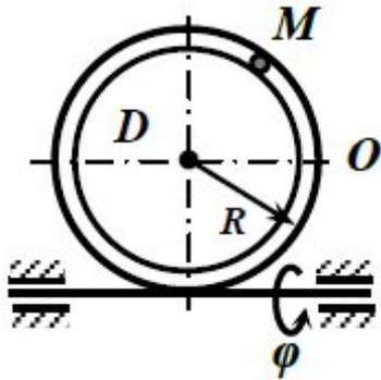
$$\varphi = t - 0,5t^3, S = 10\sqrt{2}\pi \cdot \cos 2\pi t, t_1 = 1/8 \text{ с}, R = 30 \text{ см.}$$
