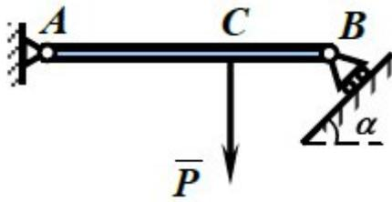
$P = 4 \text{ кН}, AB = 3 \text{ м}, AC = 2 \text{ м}, \alpha = 45^\circ.$
