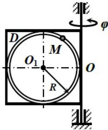
$$\varphi = 3t - 0,5t^3, S = 40\pi \cos \frac{\pi t}{6}, t_1 = 2 \text{ с}, R = 30 \text{ см.}$$
