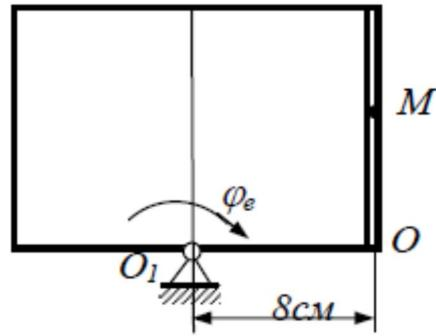
$$S_r = 8 t^2 \text{ см}, \quad \varphi_e = 4 t^2, \\ t = 1 \text{ с}$$
