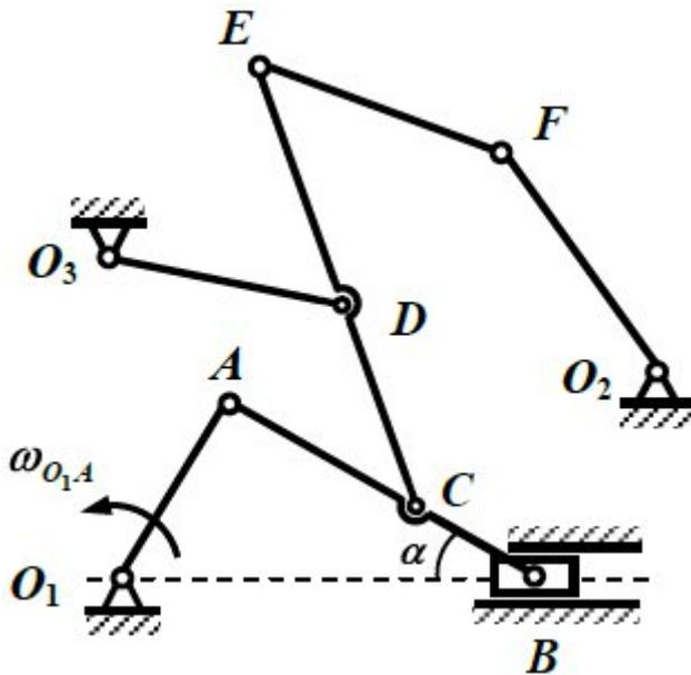
$$O_1A = 21 \text{ см}, \omega_{O_1A} = 2 \text{ рад/с}, \angle O_1AB = 90^\circ, \alpha = 30^\circ.$$
