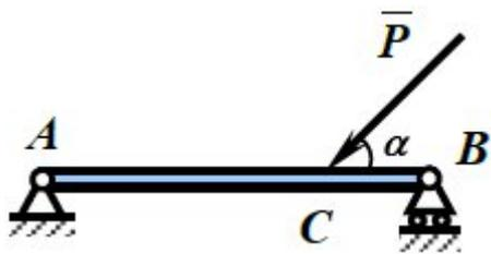
$P = 6 \text{ кН}$ ,  $AB = 4 \text{ м}$ ,  $AC = 3 \text{ м}$ ,  $\alpha = 45^\circ$ .
