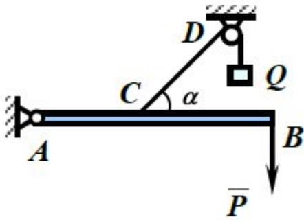
$P = 3 \text{ кН}, AB = 2 \text{ м}, AC = 1 \text{ м}, \alpha = 45^\circ.$
