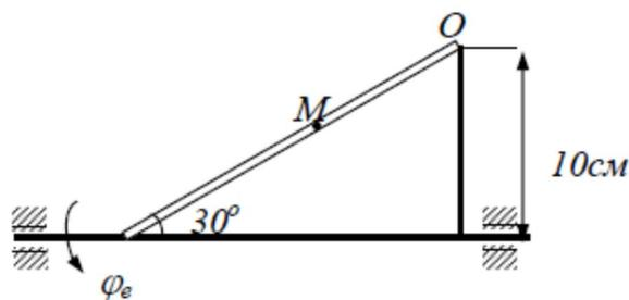
$$S_r = (15t - t^2) \text{ см}, \quad \varphi_e = 3t^2 - 4t^3, \quad t = 1 \text{ с}$$
