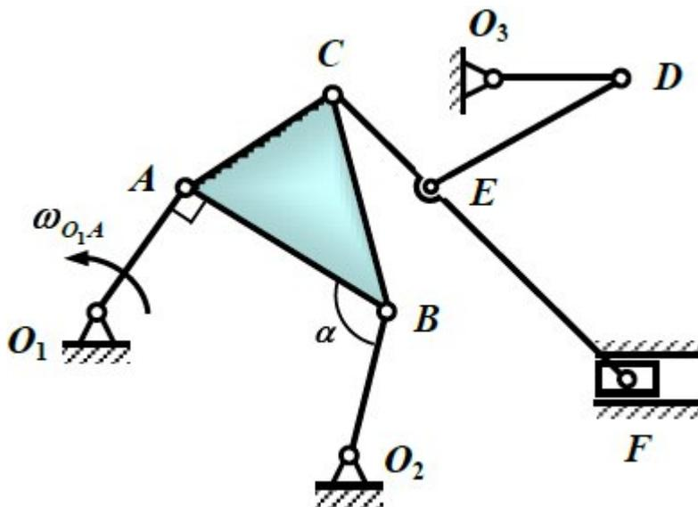
$O_1A = 15 \text{ см}, \omega_{O_1A} = 2 \text{ рад/с}, \angle O_1AB = 90^\circ, \alpha = 105^\circ.$
