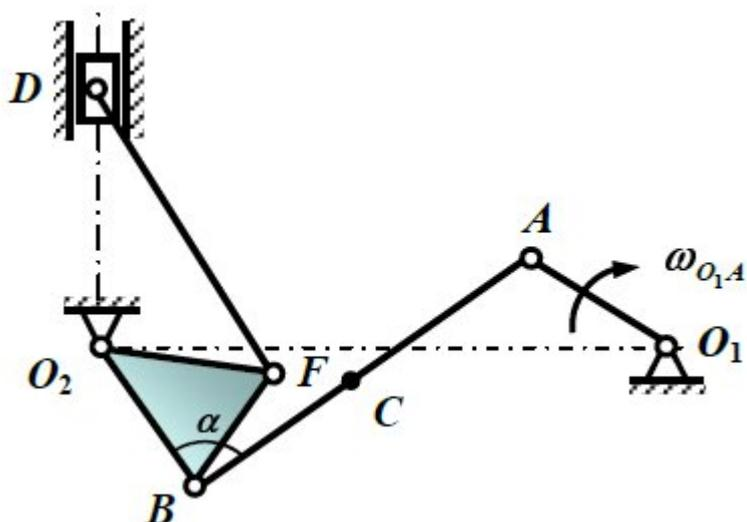
$O_1A = 15 \text{ см}, \omega_{O_1A} = 2 \text{ рад/с}, \angle O_1AB = 120^\circ, \alpha = 60^\circ.$
