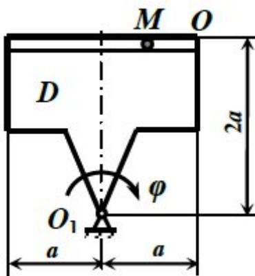
$$\varphi = 2t + 0,5t^2, S = 6t^3, t_1 = 2 \text{ с}, a = 30 \text{ см.}$$
