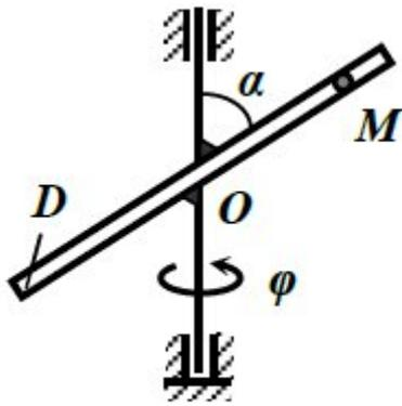
$$\varphi = 0,6t^2, S = 10\sin\frac{\pi t}{6}, t_1 = 1 \text{ с}, \alpha = 60^\circ.$$
