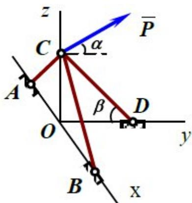
$P = 6 \text{ кН}$ ,  $\alpha = 30^\circ$ ,  $\beta = 60^\circ$ .
