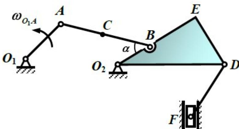
$$O_1A = 20 \text{ см}, \omega_{O_1A} = 3 \text{ рад/с}, \angle O_1AB = 120^\circ, \alpha = 45^\circ.$$
