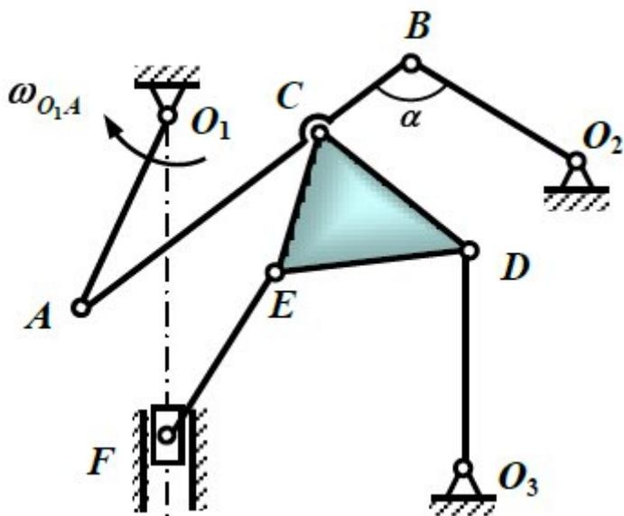
$$O_1A = 30 \text{ см}, \omega_{O_1A} = 2 \text{ рад/с}, \angle O_1AB = 30^\circ, \alpha = 120^\circ.$$
