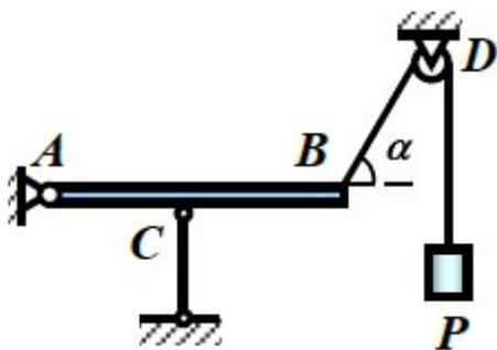
$P = 2 \text{ кН}$ ,  $AB = 2 \text{ м}$ ,  $AC = 1 \text{ м}$ ,  $\alpha = 60^\circ$ .
