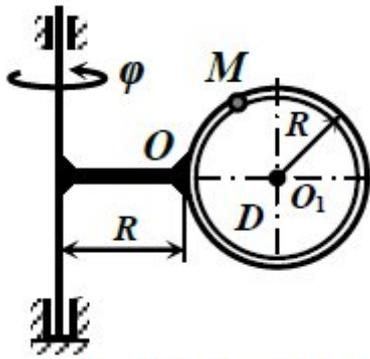
$$\varphi = 1,2t - t^2, S = 20\pi \cos \frac{\pi t}{4}, t_1 = \frac{4}{3} \text{ с}, R = 20 \text{ см.}$$
