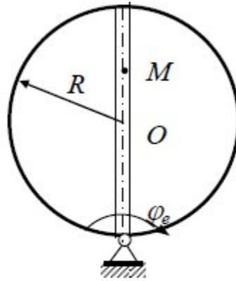
$$S_r = 20 \sin(\pi t/3) \text{ см}, \quad \varphi_e = 6t - 2t^3, \\ t = 0,5 \text{ с}, \quad R = 20 \text{ см}.$$
