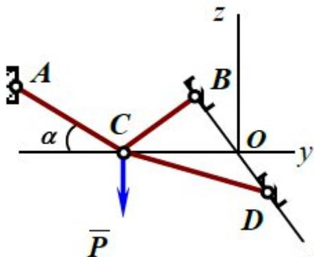
$P = 5 \text{ кН}$ ,  $\alpha = 30^\circ$ ,  $AC \perp Ox$ ,  $OB = OD = OC$
