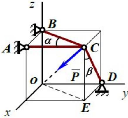
$P = 2 \text{ кН}, \alpha = 30^\circ, \beta = 60^\circ, AB = a$
